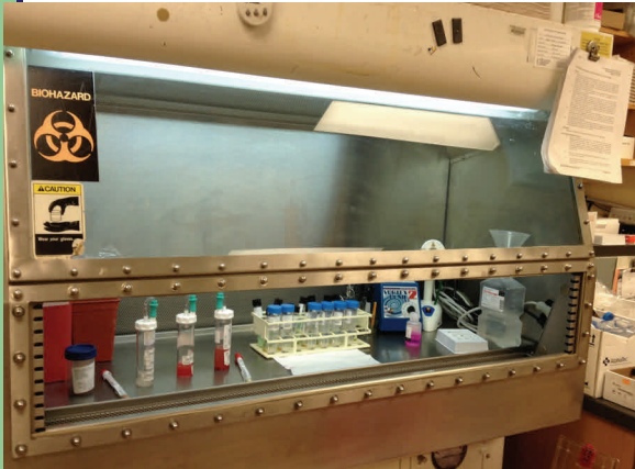
Above: Acid fast Biosafety cabinet with row of specimens being digested
