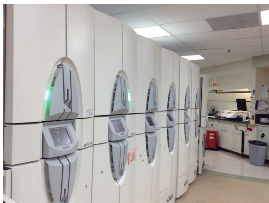
Above: Row of Bactec blood culture instruments. SSM has capacity for 2600 blood culture bottles and receive approximately 150 blood culture sets per day.
